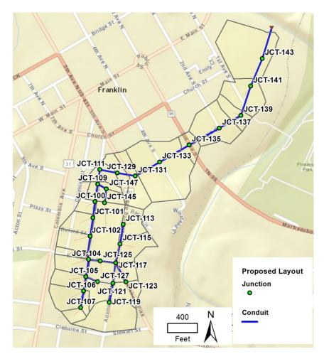
Figure 6: Proposed Storm Sewer Layout
