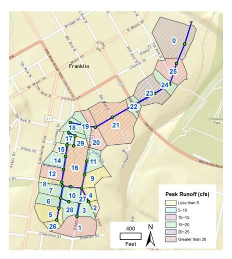
Figure 7: Subbasins Maximum Discharge
