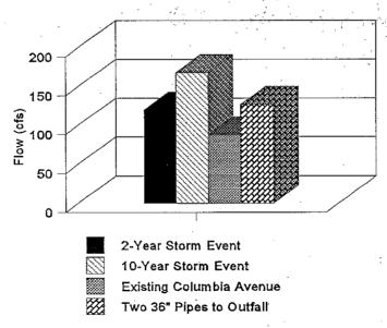
Based upon the above graph, it becomes evident that the existing drainage ways under Columbia Avenue can not pass the 2- or 10-year storm events. After performing the investigation and finding that the critical section is under Columbia Avenue, we investigated the following options. Option 1 is to install a storm sewer system which would encompass the entire Parkview drainage area as
