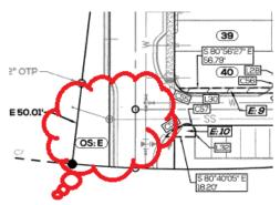
The sanitary sewer easement for the servioce to the body shop must be a minimum of 20' easement for maintenance.
