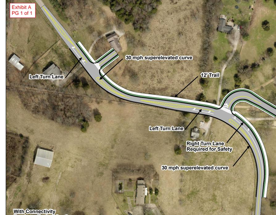
With Connectivity Two Lane Typical Section Design Speed = 40 mph Posted Speed = 30 mph
