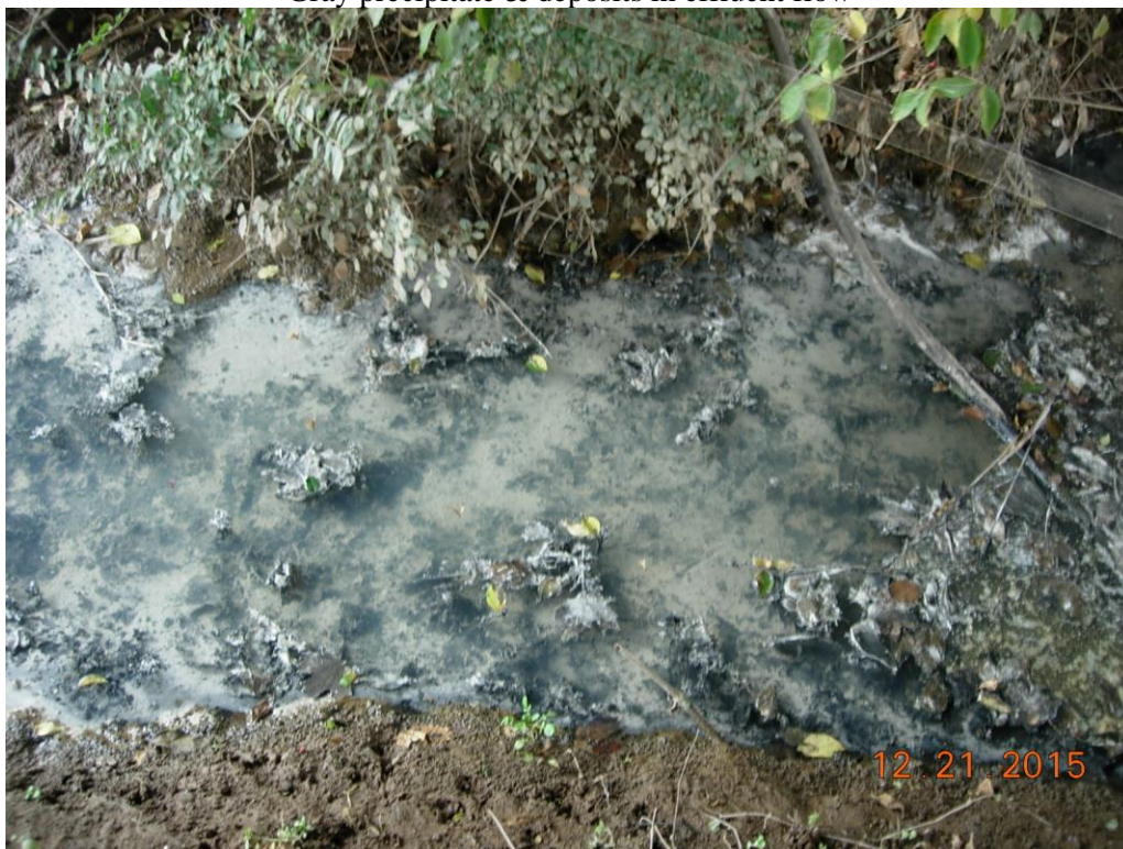
Gray & blackish precipitate & deposits in effluent flow
