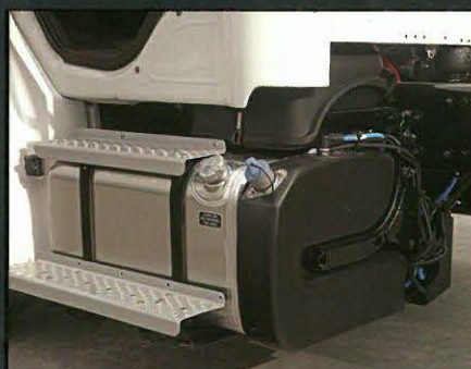
Up to two batteries located under cab for easy body upfit.
