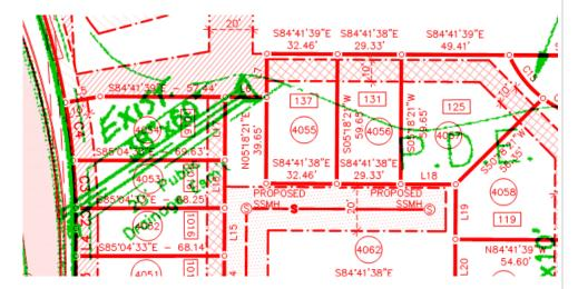
The call-out for the proposed drainage easement around the portion of Lake Westhaven adjacent to the condos shall be revised to remove the "along 642' contour" portion of the text. The original easement around the lake was based on the 642' contour, but that is to be revised for the portion adjacent to the condos and commercial site where revised grading has changed the easement line. The line appears to be drawn correctly from the site plan, but does not follow the 642' contour in this area.
