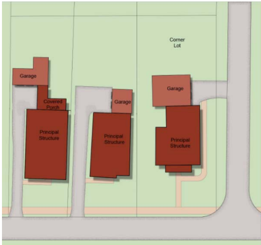
Figure 5-7: These examples show how attached garages are traditionally placed and subordinate to the rest of the principal structure.
