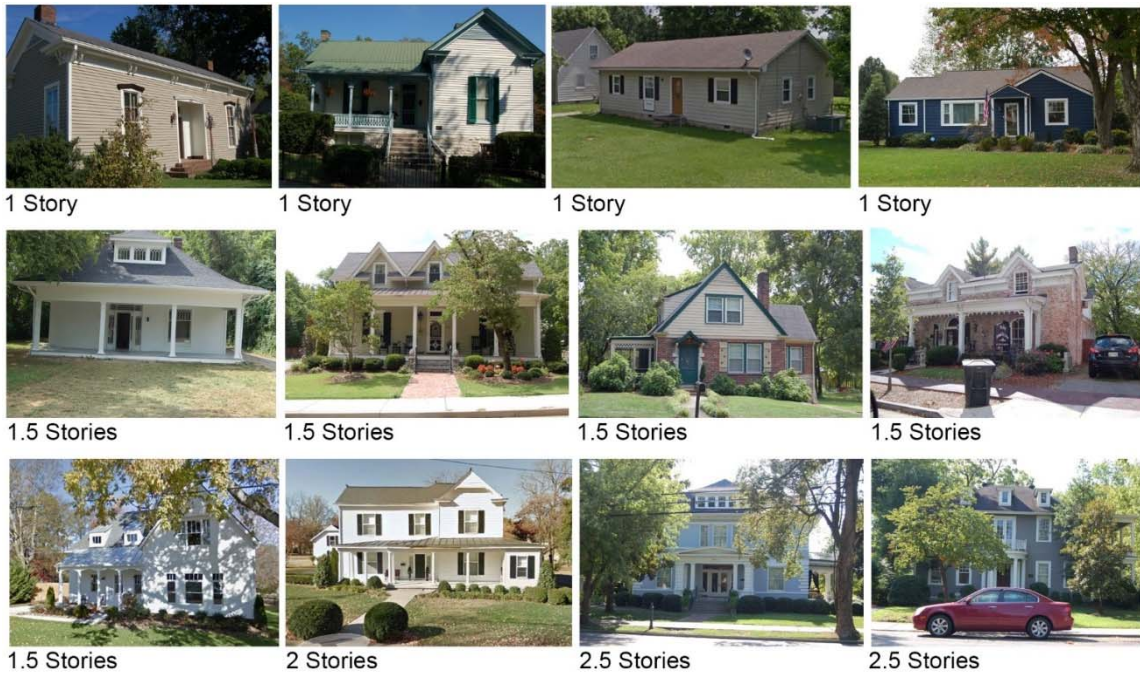
Figure 5-5: These examples depict whole and half-stories for the purposes of determining building height.
