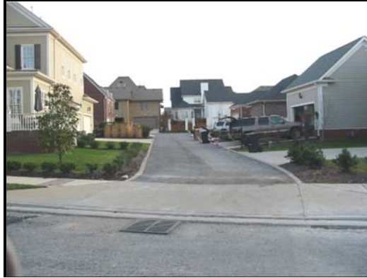
Residential Alleys Allow Service Functions to Occur at the Rear of Dwellings and Reduce the Impact of Cars, Driveways and Garage Doors on Streets Figure 3.3 (1)
