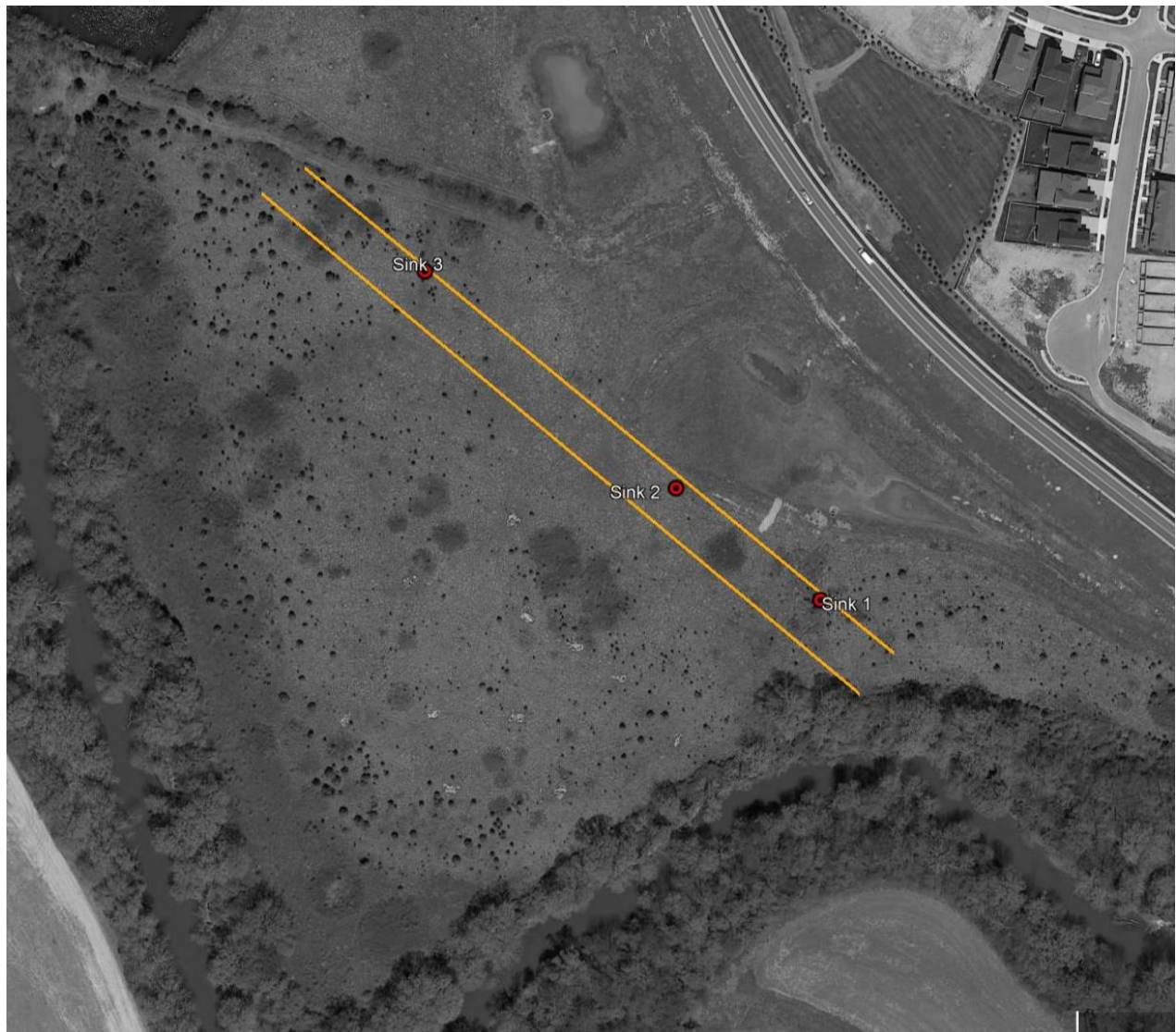
Figure 1b – Geophysical Test Lines in park area to investigate sinkholes
