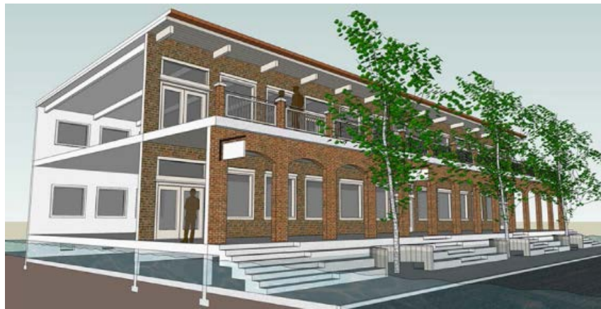
Figure 3-17. Conceptual model of low-rise nonresidential building above the Base Flood Elevation, along the southern half of the block.
