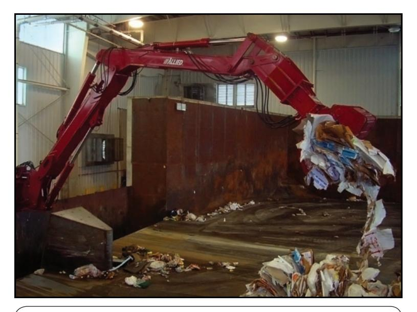
Allied Construction Products, LLC has developed a new Pedestal Transfer Boom System specifically for the waste transfer industry. It offers consistent reliability and high productivity for lowering waste handling costs. And, it's backed by decades of Allied experience in designing and building Pedestal Transfer Boom Systems for other demanding applications.
