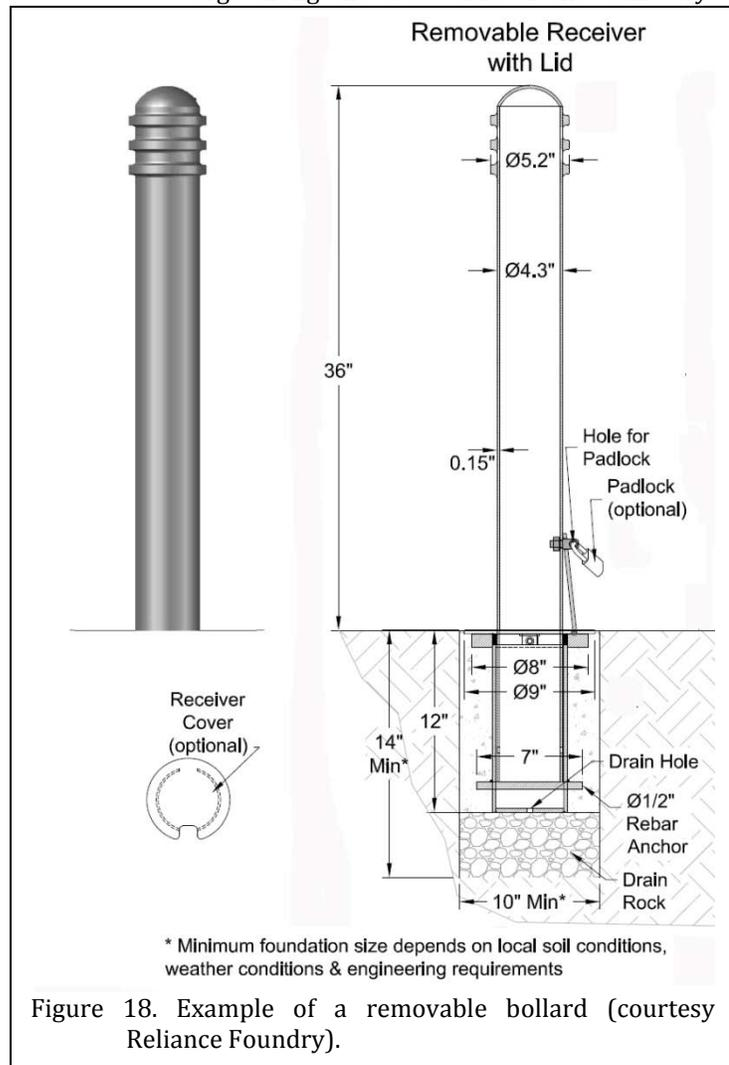
Figure 18. Example of a removable bollard (courtesy Reliance Foundry).
