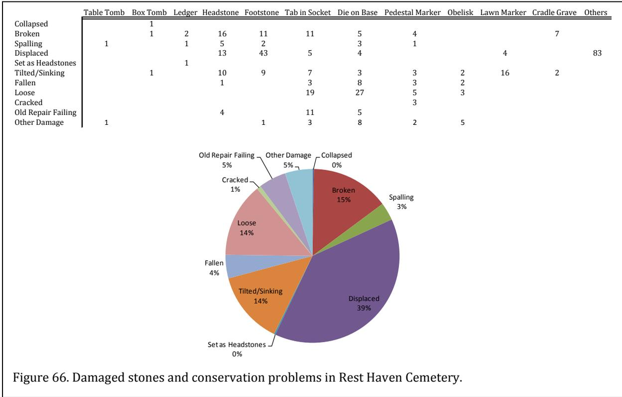
Figure 66. Damaged stones and conservation problems in Rest Haven Cemetery.
